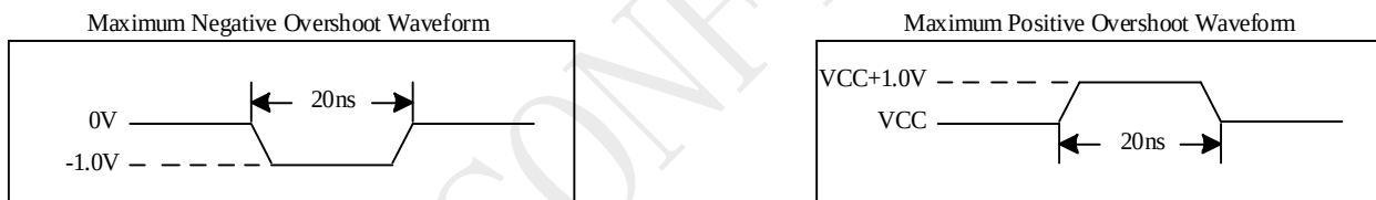
Figure 5-3 Maximum Overshoot Waveform
