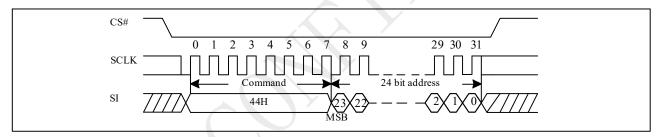
Figure 10-46a Erase Security Registers (ERSCUR) Sequence (QPI)
