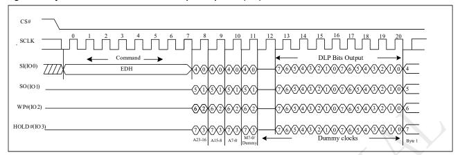
Note: The DLP bit is also valid for 4-byte EDH and EEH instruction and QPI 4IO DTR read instruction.
