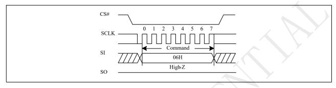
Figure 10-2a Write Enable (WREN) Sequence (QPI)
