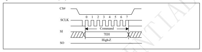
Figure 10-62a Global Block Lock (QPI)
