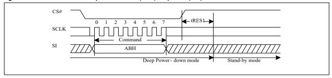
Figure 10-50c Release from Deep Power-down (RDP) Sequence (QPI)
