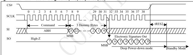
Figure 10-50a Read Electronic Signature (RES) Sequence (QPI)
