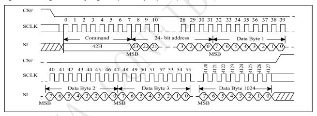
Figure 10-47a Program Security Registers (PRSCUR) Sequence (QPI)
