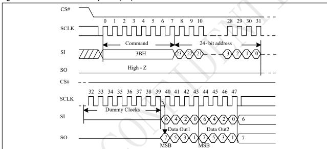
Figure 10-18 Dual Read Mode Sequence (SPI)
