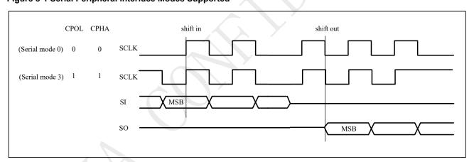
Figure 8-1 Serial Peripheral Interface Modes Supported
