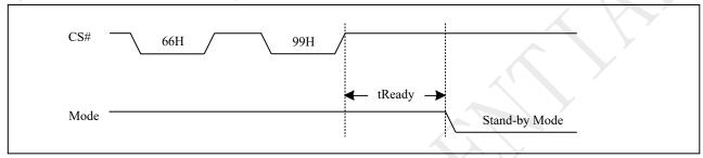
Figure 10-64a Software Reset Sequence (SPI)
