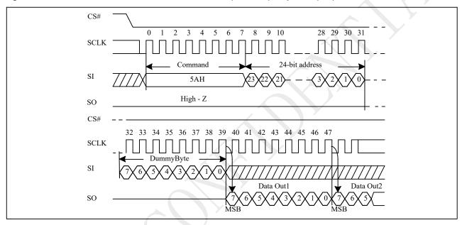
Figure 10-68a Read Serial Flash Discoverable Parameter (RDSFDP) Sequence (QPI)
