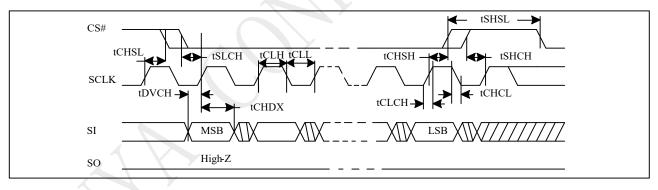
Figure 5-5 Output Timing
