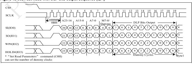
Figure 10-30a Fast Read with DLP bits output Sequence (QPI)
