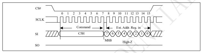
Figure 10-10a Write Extended Address Register Sequence (QPI)
