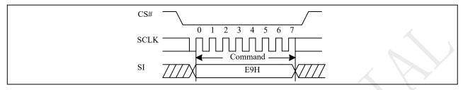
Figure 10-12a Exit 4-Byte Address Mode Sequence (QPI)
