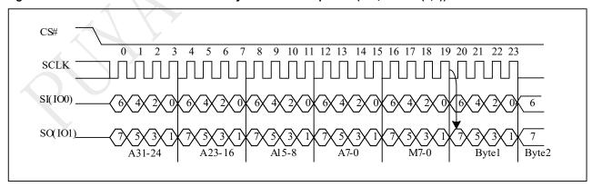
Note:2IO Continue Read with 4-Byte Address, if M5-4 = 1, 0. If not using Continue Read recommend to set M5-4  $\neq$  1, 0.
