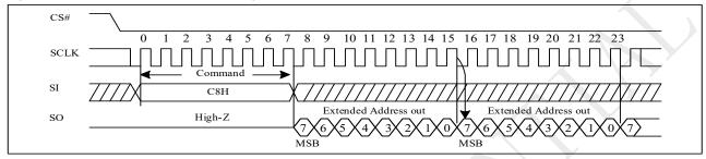
Figure 10-9a Read Extended Address Register Sequence (QPI)
