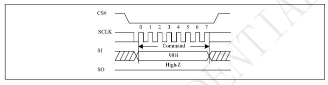
Figure 10-63a Global Block Unlock (QPI)
