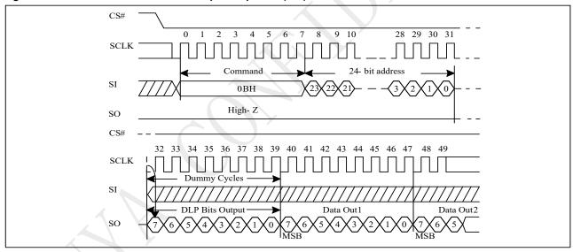
Figure 10-30 Fast Read with DLP bits output Sequence (SPI)
