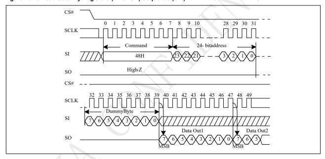
Figure 10-48a Read Security Registers (RDSCUR) Sequence (QPI)
