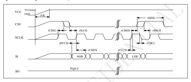
Figure 5-9 Power-up Timing
