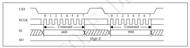
Figure 10-64b Software Reset Sequence (QPI)
