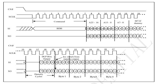
Figure 9-23I DTR 4IO Read with DLP bits output Sequence
