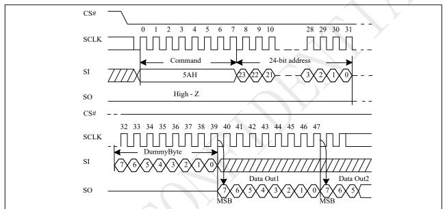
Figure 9-53 Read Serial Flash Discoverable Parameter (RDSFDP) Sequence
