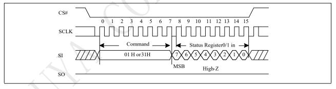
Figure 9-7 Write Status Register (WRSR) Sequence (Command 01h or 31h)
