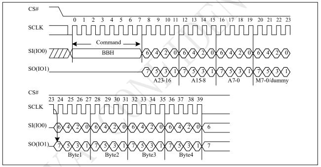
Figure 9-13 2IO Read Sequence (Command BBh M5-4 ≠ (1,0))
