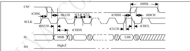
Figure 5-5 Output Timing
