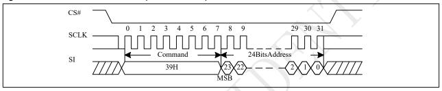
Figure 10-51a Individual Block Unlock(QPI)
