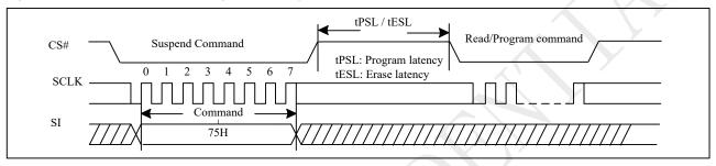
Figure 10-48a Suspend to Read/Program Latency(QPI)
