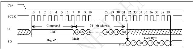
Figure 10-52a Read Block Lock Status (QPI)
