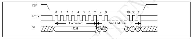
Figure 10-28a Block Erase 32K(BE32K) Sequence (QPI)
