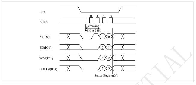
Figure 10-7b Write Status Register (WRSR) Sequence (Command 01)
