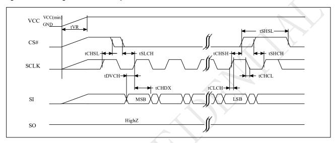
Figure 5-9 Power-up Timing
