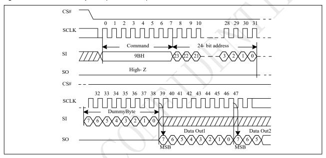
Figure 10-35a Buffer Read Sequence (QPI)
