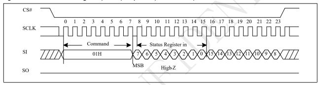
Figure 10-7c Write Status Register (WRSR) Sequence (QPI)
