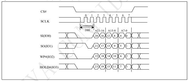
The self-timed Sector Erase Cycle time (tSE) is initiated as soon as Chip Select (CS#) goes high. The Write in progress (WIP) bit still can be check out during the Sector Erase cycle is in progress. The WIP sets 1 during the tSE timing, and sets 0 when Sector Erase Cycle is completed, and the Write Enable Latch (WEL) bit is reset. If the sector is protected by BP4, BP3, BP2, BP1, BP0 bits, the Sector Erase (SE) instruction will not be executed on the sector.
