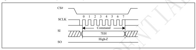
Figure 10-53a Global Block Lock(QPI)
