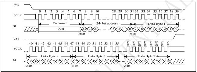
Figure 10-36a Buffer Write Sequence (QPI)
