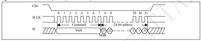
Figure 10-34a Buffer Load Sequence (QPI)
