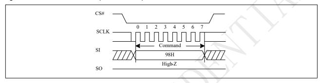
Figure 10-54a Global Block Unlock(QPI)
