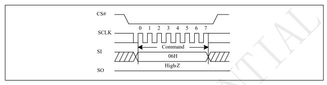
Figure 10-2a Write Enable (WREN) Sequence (QPI)
