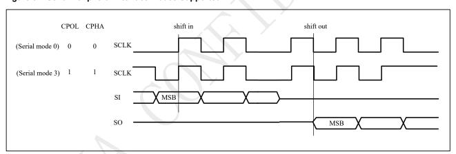
Figure 8-1 Serial Peripheral Interface Modes Supported
