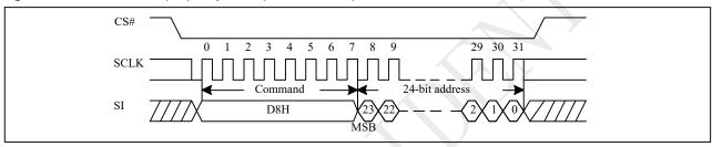
Figure 10-29a Block Erase (BE) Sequence (QPI)
