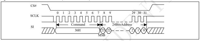
Figure 10-50a Individual Block Lock(QPI)
