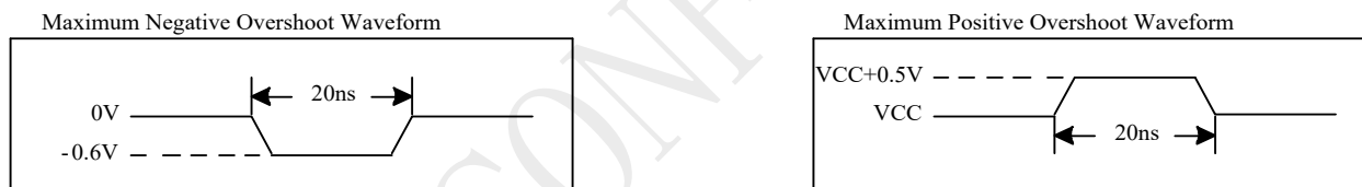
Figure 5-3 Maximum Overshoot Waveform
