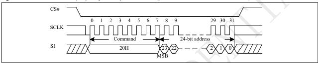
The self-timed Sector Erase Cycle time (tSE) is initiated as soon as Chip Select (CS#) goes high. The Write in progress (WIP) bit still can be check out during the Sector Erase cycle is in progress. The WIP sets 1 during the tSE timing, and sets 0 when Sector Erase Cycle is completed, and the Write Enable Latch (WEL) bit is reset. If the sector is protected by BP4, BP3, BP2, BP1, BP0 bits, the Sector Erase (SE) instruction will not be executed on the sector.
