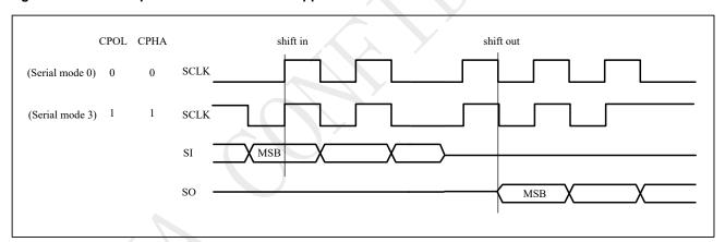
Figure 8-1 Serial Peripheral Interface Modes Supported
