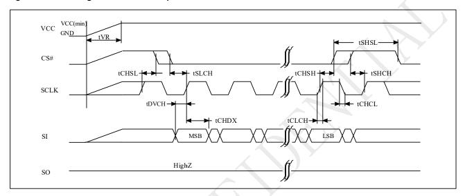
Figure 5-9 Power-up Timing
