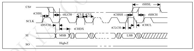
Figure 5-5 Output Timing
