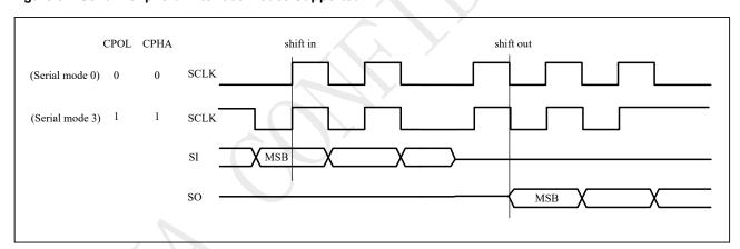
Figure 8-1 Serial Peripheral Interface Modes Supported
