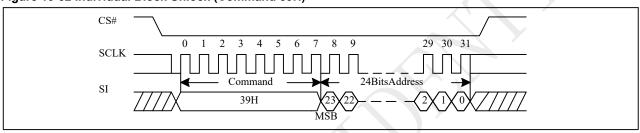
Figure 10-52a Individual Block Unlock(QPI)
