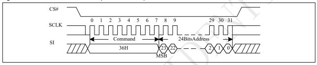
Figure 10-51a Individual Block Lock(QPI)
