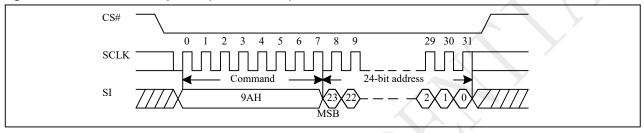
Figure 10-34a Buffer Load Sequence (QPI)
