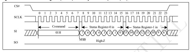
Figure 10-7b Write Status Register (WRSR) with 2 Byte data Sequence (QPI)
