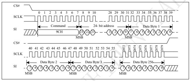
Figure 10-36a Buffer Write Sequence (QPI)
