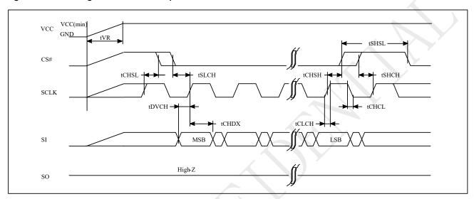
Figure 5-9 Power-up Timing
