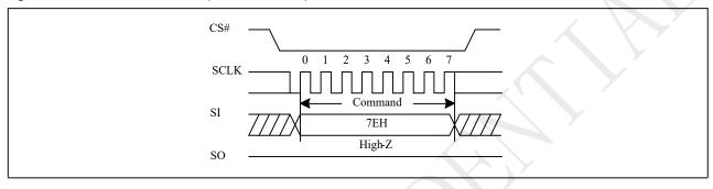
Figure 10-54a Global Block Lock(QPI)
