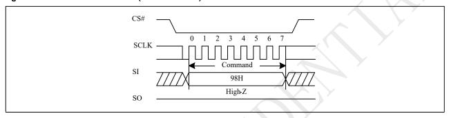
Figure 10-55a Global Block Unlock(QPI)
