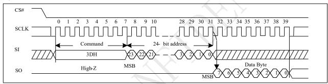
Figure 10-53a Read Block Lock Status (QPI)
