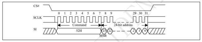
Figure 10-28a Block Erase 32K(BE32K) Sequence (QPI)
