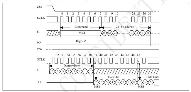
Figure 10-35a Buffer Read Sequence (QPI)
