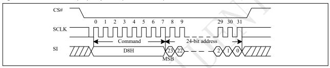
Figure 10-29a Block Erase (BE) Sequence (QPI)
