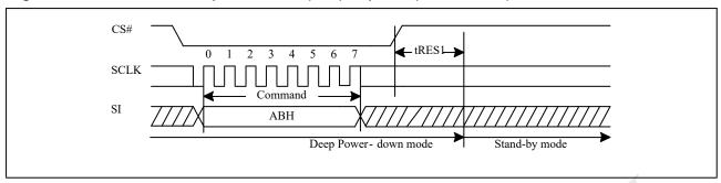
Figure 10-42c Release from Deep Power-down (RDP) Sequence (QPI)
