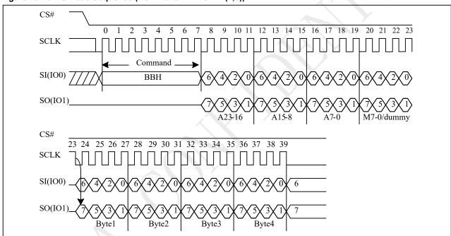
Figure 10-13 2IO Read Sequence (Command BB M5-4 ≠ (1,0))
