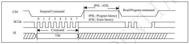
Figure 10-48a Suspend to Read/Program Latency(QPI)
