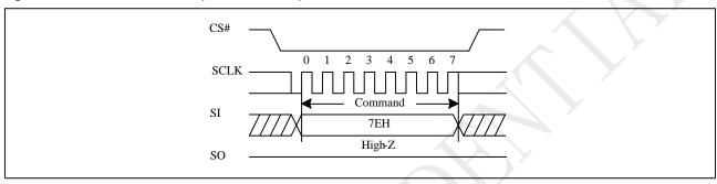
Figure 10-54a Global Block Lock(QPI)
