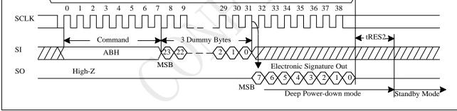
Figure 10-42a Read Electronic Signature (RES) Sequence (QPI)
