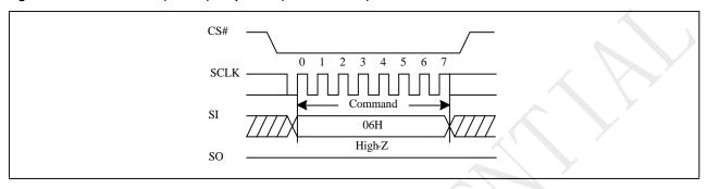
Figure 10-2a Write Enable (WREN) Sequence (QPI)
