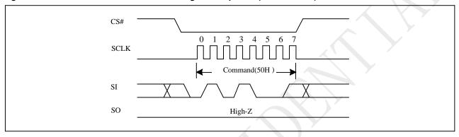
Figure 10-4a Write Enable for Volatile Status Register Sequence (QPI)
