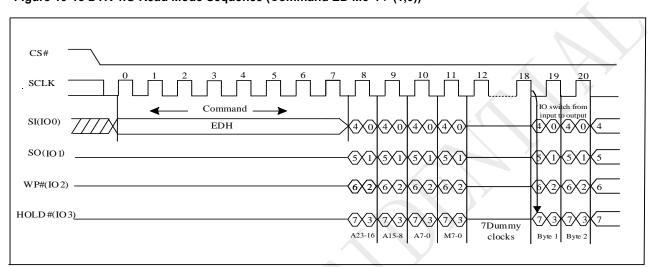
Figure 10-18 DTR 4IO Read Mode Sequence (Command ED M5-4 ≠ (1,0))
