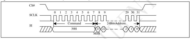
Figure 10-52a Individual Block Unlock(QPI)
