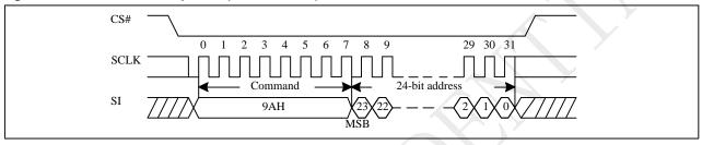
Figure 10-34a Buffer Load Sequence (QPI)
