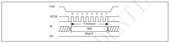
Figure 10-55a Global Block Unlock(QPI)
