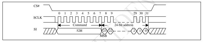
Figure 10-28a Block Erase 32K(BE32K) Sequence (QPI
