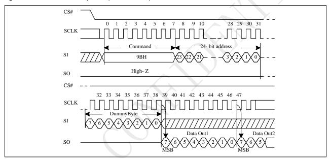
Figure 10-35a Buffer Read Sequence (QPI)
