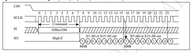
Figure 10-5a Read Status Register (RDSR) Sequence (QPI)
