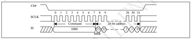
Figure 10-29a Block Erase (BE) sequence (QPI)
