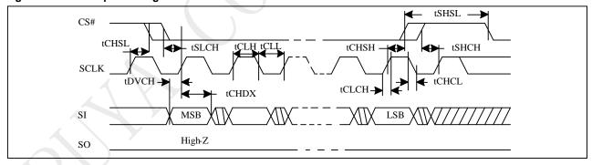
Figure 5-5 Output Timing
