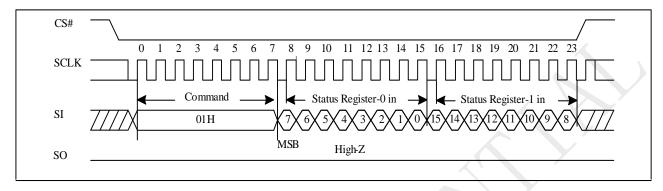
Figure 10-7C Write Status Register (WRSR) with 2 Byte data Sequence (QPI)
