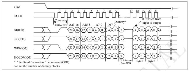
Figure 10-23e DTR 4IO Read with DLP bits output Sequence
