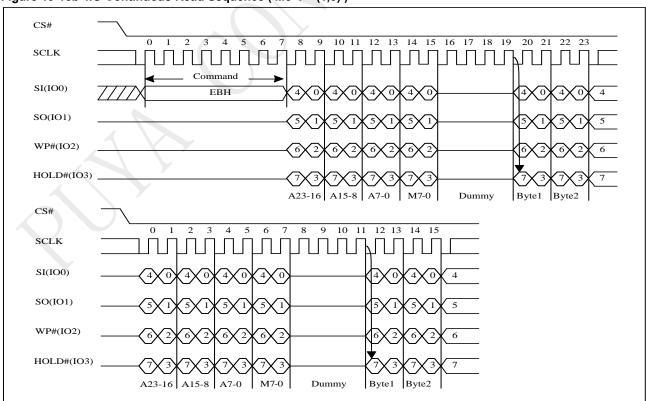
Note: 4IO Continuous Read Mode, if M5-4 = 1, 0. If not using Continuous Read recommend to set M5-4  $\neq$  1, 0.
