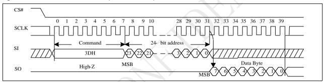
Figure 10-53a Read Block Lock Status (QPI)
