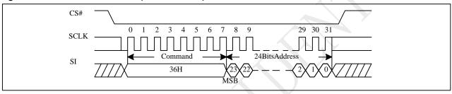
Figure 10-51a Individual Block Lock(QPI)
