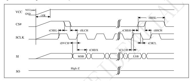
Figure 5-9 Power-up Timing
