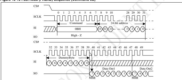
Figure 10-10 Fast Read (FREAD) Sequence (Command 0B)
