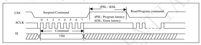
Figure 10-48a Suspend to Read/Program Latency(QPI)
