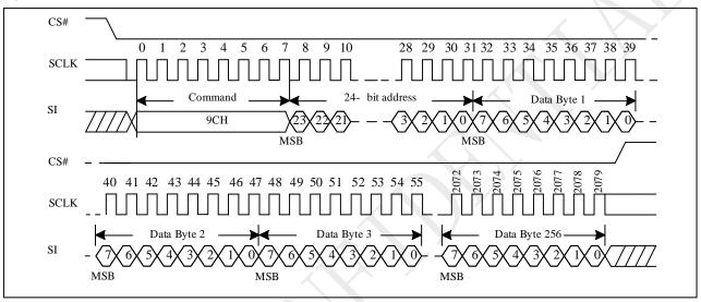
Figure 10-36a Buffer Write Sequence (QPI)
