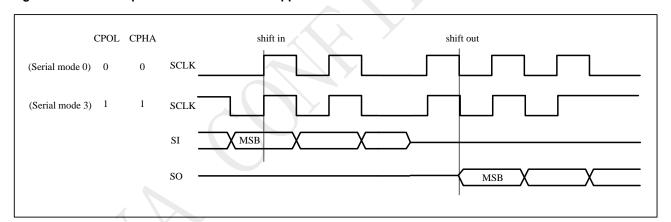
Figure 8-1 Serial Peripheral Interface Modes Supported
