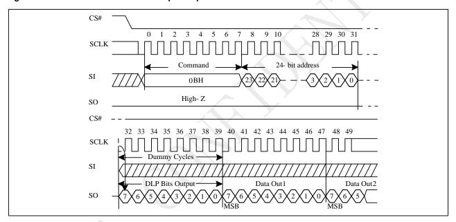
Figure 10-23a Dual Read with DLP bits output Sequence
