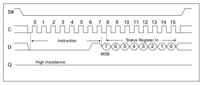
Driving the Chip Select (S#) signal high at a byte boundary of the input data triggers the self-timed Write cycle
