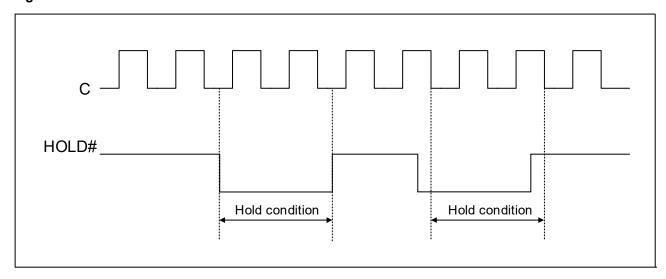
The Hold condition starts when the Hold (HOLD#) signal is driven low when Serial Clock (C) is already low (as shown in Figure 5-1).
