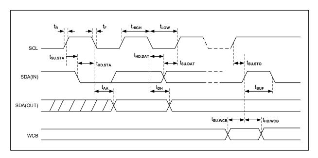
Figure 3-2 Write Cycle Timing
